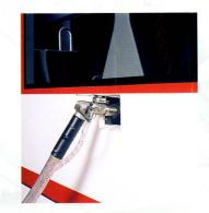
With the filling valve inserted into the sand boxand the sanding system switched on, the sand flow automatically stops when the filling level of the sand box is reached - much like filling your gas tank at the filling station.
