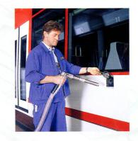
The sand filling process is smooth. In order to prevent sand from being spilled outside the sand box, the filling valve is equipped with a segmental lock. Thanks to the special design of the vent connection, only dust is extracted but no sand.
