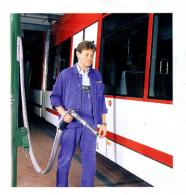
The ergonomically designed filling valve with sealing cone, which distinguishes itself by easy handling, ensures a dust-free connection to the sand box and is almost universally applicable.
