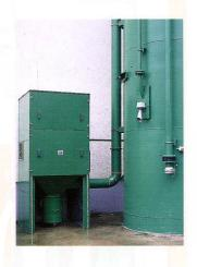
For health reasons it is recommended to dispose of lung piercing silica dust at only one point of the sanding plant. The automatic air return system carries the dust from the individual filling valves to a central filter by means of a special injector system Here, the dust can be disposed of without harming the environment.
